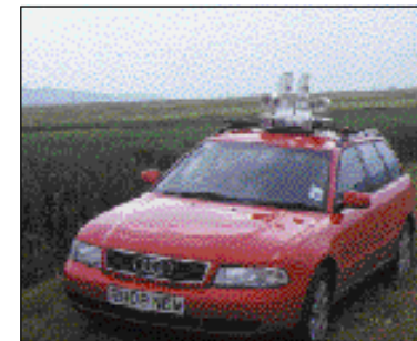
Wind impaction spore trap on a car roof. This is used, especially for Blumeria graminis , to conduct surveys to monitor the development and status of fungicide resistance. (Syngenta)
