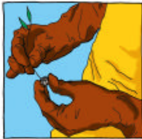
Do not blow out clogged nozzles with the mouth—clean them with water or a soft probe
