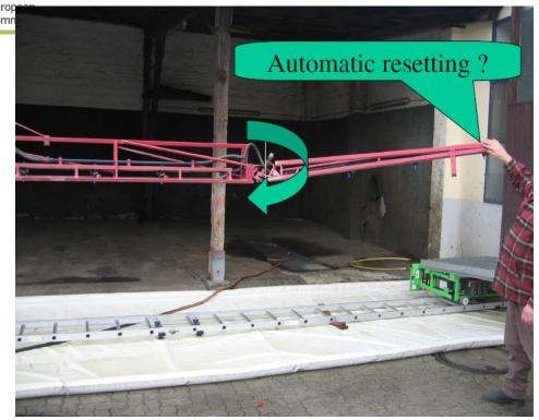
4.8.1 The boom shall be stable in all directions, i.e. not loose in any joints and not be bent.
