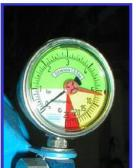
The scale shall be marked: <5 bar: 0,2 bar 5-20bar: 1,0 bar >20 bar: 2,0 bar
