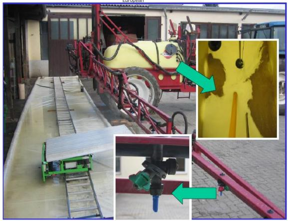
b) the pump shall have sufficient flow rate capacity in order to be able to spray at maximum working pressure as recommended by the sprayer or the nozzle manufacturer during test with the largest nozzles mounted on the boom while maintaining a visible agitation as specified in 4.3:—
