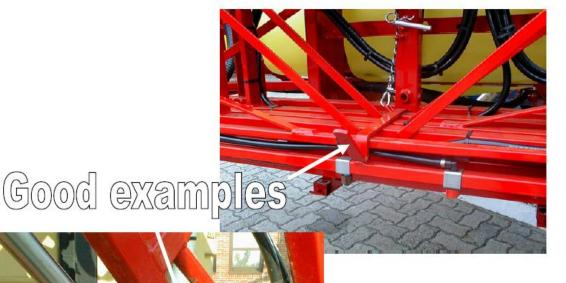
4.8.3 The boom shall be securely lockable in the transport position.
