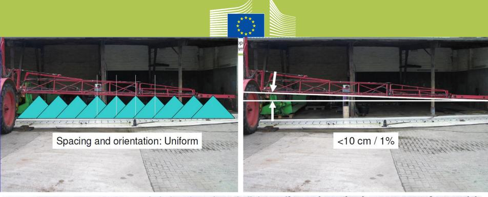
**4.8.4** The nozzle spacing and their orientation shall be uniform along the boom, except for special equipment such as border spraying. By design, it shall not be possible to modify unintentionally the position of the nozzles in working conditions, for example by folding/unfolding the boom.
