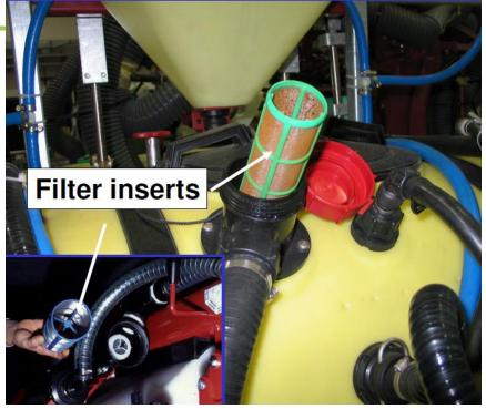
4.7.2 If an isolating device is provided, it shall be possible, with the tank filled to its nominal volume, to clean filters without any spray liquid leaking out except for that which may be present in the filter casing and the suction lines.
