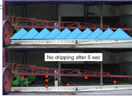
4.9.1 All nozzles shall be identical (type, size, material and origin) all along the boom, except where they are intended for a special function for example the end nozzles for border spraying.
