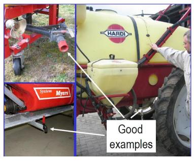
4.4.5 There shall be a clearly readable liquid level indicator on the tank which is visible from the driver's position and from where the tank is filled.
