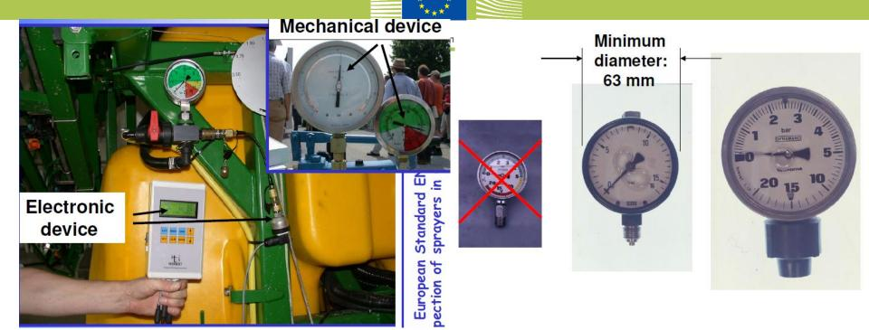
4.5.5 For analogue pressure gauges the minimum diameter of the pressure gauge cases shall be 63 mm.
